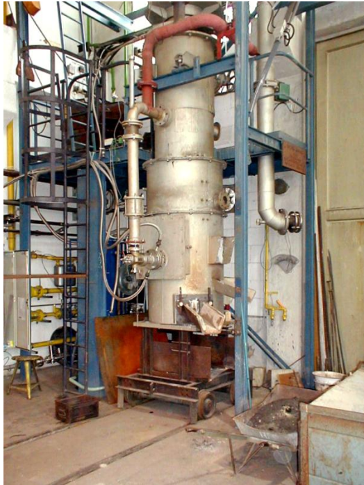
Fig. 2: Cupola furnace plant for melt-gassing in pilot plant scale, © Ingitec 2009
